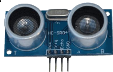
Figure 14. Ultrasonic transceiver HR-SR04
